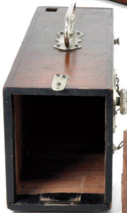
The plate rack that held the ferrotypes was inverted open side down before loading into the back of the Nodark
