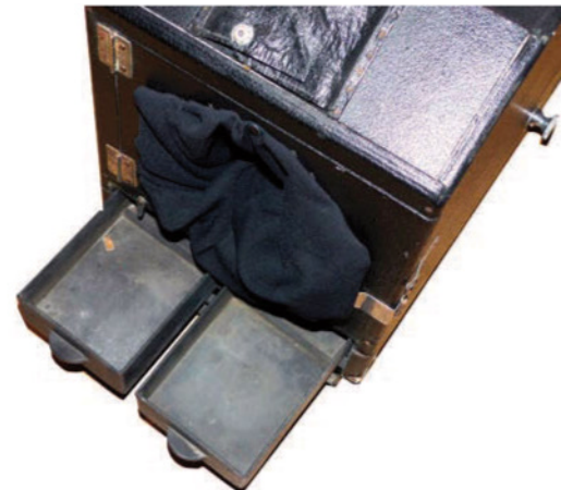
The twin drawers in the back of the Jano which contained developer and fixer and, above them, the elasticated sleeve used to manipulate items inside the camera
