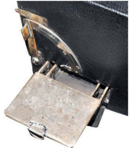
How ferrotype plates were loaded into the Aptus
