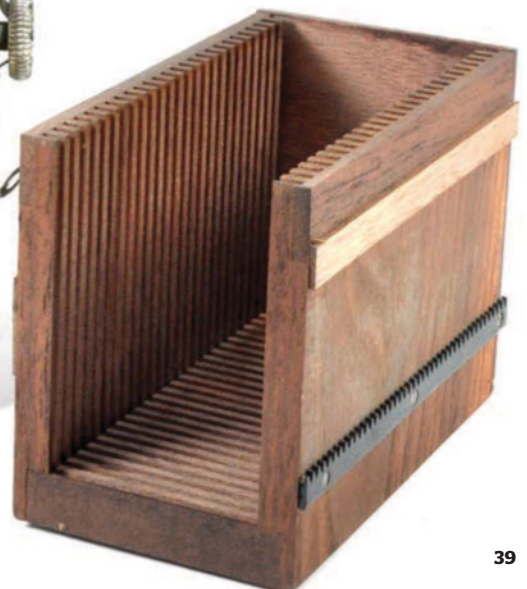
The plate rack that held the ferrotypes was inverted open side down before loading into the back of the Nodark
