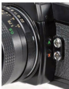
The adapter's cable plugs into a socket marked 'A' just above the traditional flash sync socket
