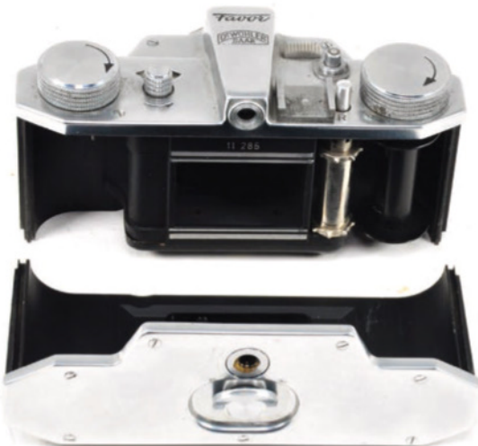
The base and back are removed in one piece for easy film loading
