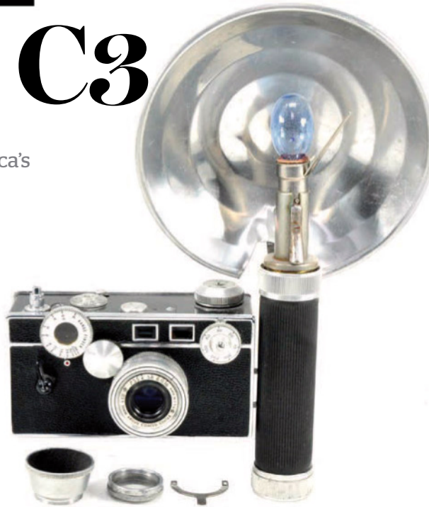
Argus C3 with its dedicated flashgun fitted and, below it, the camera's lens hood, filter and special aperture adjusting accessory
