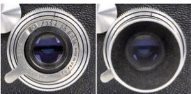
The 'Y'-shaped accessory in place on the aperture ring (left) and how the lens hood then obscured the settings
