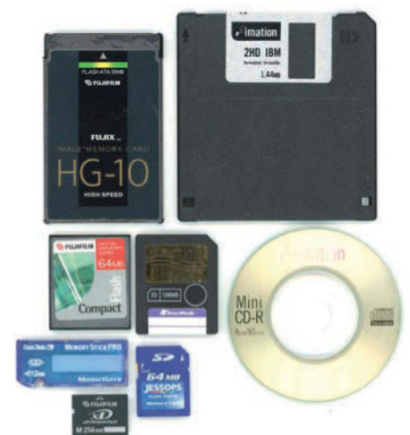
Storage devices down the digital ages: PC card, floppy disc, mini compact disc, SmartMedia card, Memory Stick card, xD Picture Card, CompactFlash and SD card
