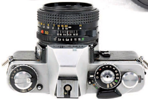
The XD7 from above shows the mode selector switch around the shutter speed dial
