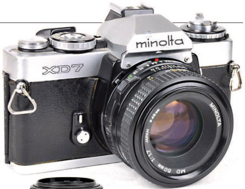
Minolta XD7, first with multi-mode exposure metering
