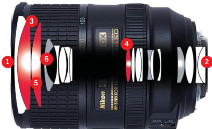
Cross-section of a Nikkor AF-S DX 18-300mm f/3.5-5.6G ED VR
