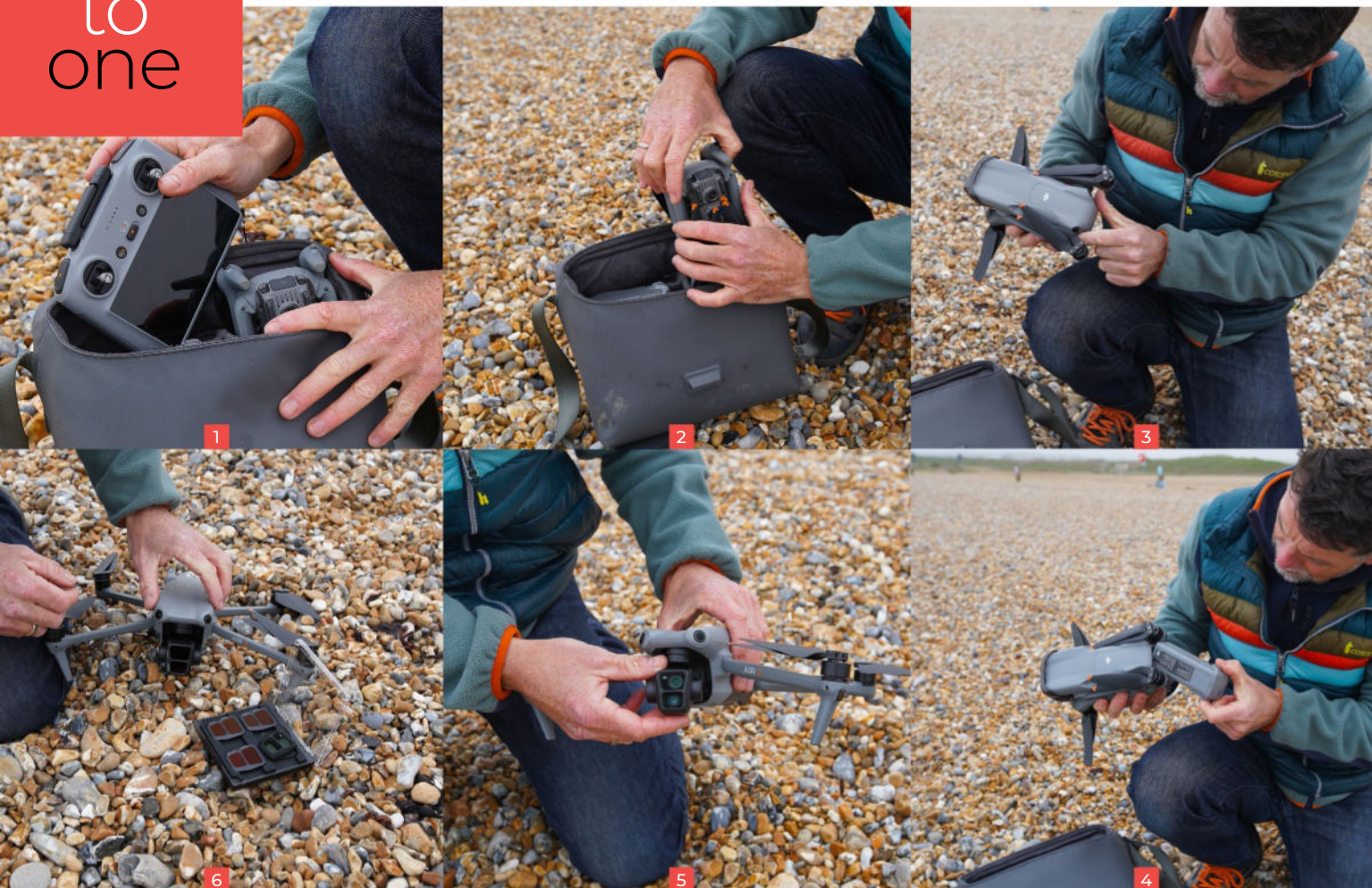
Clockwise from top left: the RC controller and DJI Air 3 stow in a small bag. Unfolding the drone and extending its propellers. Fitting the battery – Kennedy always carries spares. Preparing to fit clip-on dual ND filters, essential for filming video. Strengths range from ND8/16 to ND64/128.
