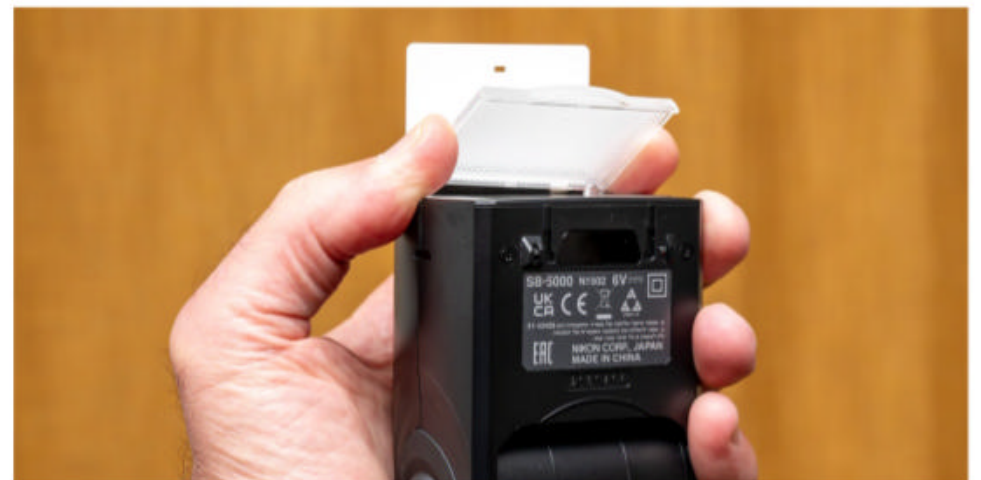
Most flashguns feature both a pull-out catchlight card and a flip-down wide-angle diffuser, to help control your scene lighting.
