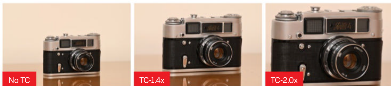
This sequence shot at the long end of a 70-200mm f/2.8 lens shows the magnification effect of no teleconverter, 1.4x giving a focal length of 280mm, and 2x with a 400mm focal length.
