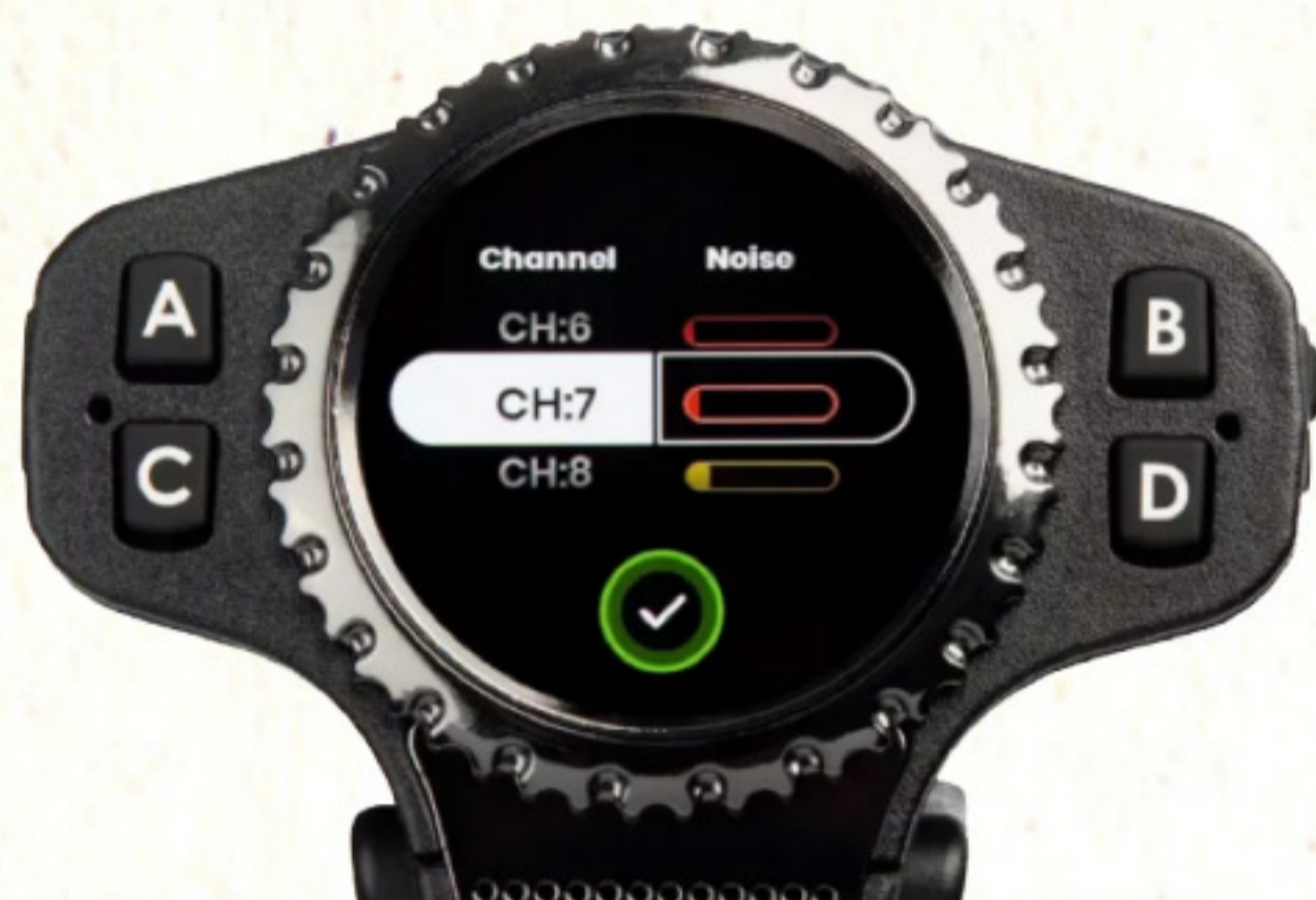
RF Noise Indicator: Find the cleanest Channel to maximize range and reliability
