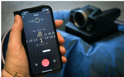
The Polaroid app automatically pairs with the I-2 when you turn it on, giving you control over modes and exposure settings, plus a self-timer countdown
