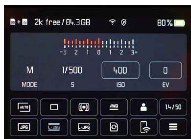
▲ Monitor-based 'Quick Menu' display/control panel offers the speed and convenience of touch screen access for both the exposure settings and the function tiles.
