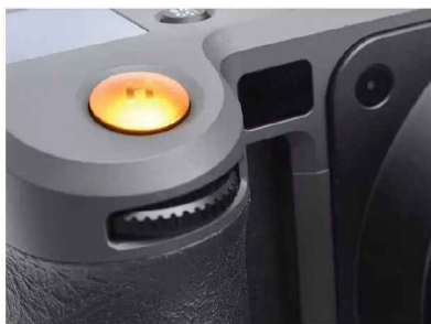
▲ AF illuminator is part of the LiDAR system for low-light assistance. Smaller window closest to the lens mount is the colour temperature sensor which assists the auto white balance measurements.
