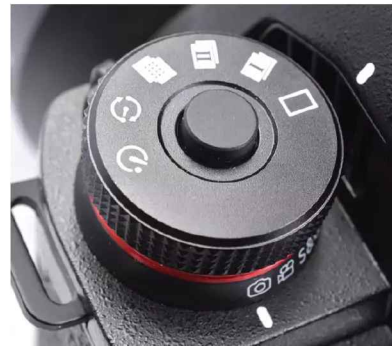
▲ Drive mode dial also engages the self-timer and the multi-shot 'High Resolution' capture function.
