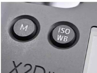
▲ Dedicated buttons for selecting exposure modes and ISO or white balance adjustments. These controls are customisable.
