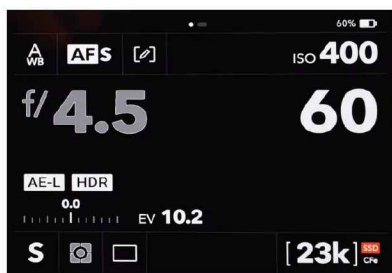
▲ Monitor-based 'Control Screen' has 'quick menu' touch for the key capture-related settings such as white balance.
