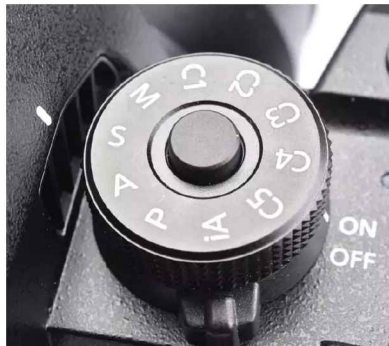
▲ Main mode dial is lockable via its central button. Note the five 'C' positions for storing customised camera set-ups.
