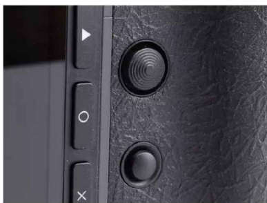
▲ Rear panel control layout now includes a five-way joystick-type controller.
