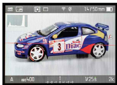
▲ Live view screen elements include a real-time histogram, guide grids and dual-axis level indicator. You can have them all in one display or in separate displays and, of course, in both the EVF and the monitor. Focus peaking in red is also shown here.
