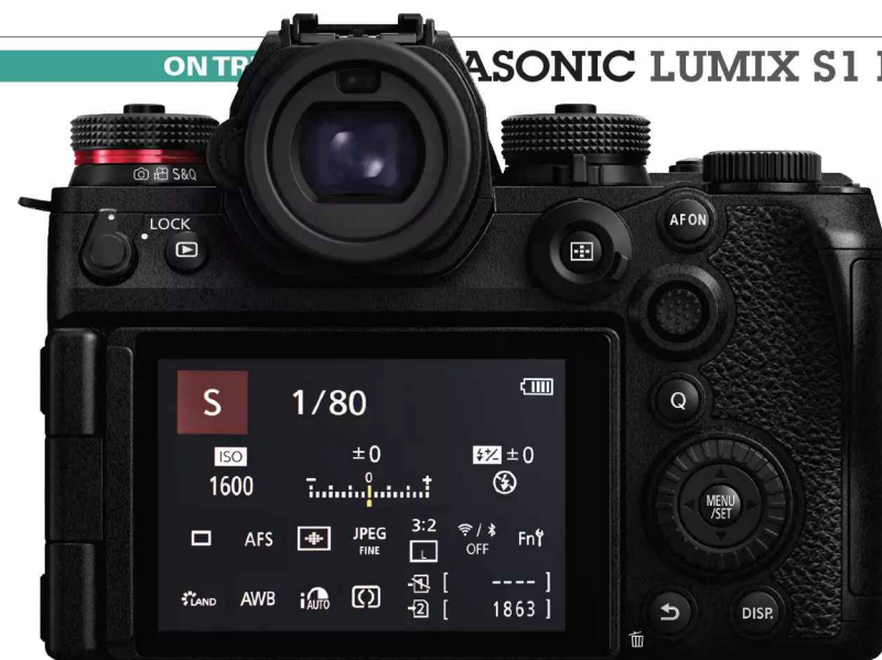
▲ Rear panel control layout includes a joystick controller and a control wheel with four-way navigational actions. Bodysell is magnesium alloy – covers and chassis – with weather sealing and insulation for shooting in subzero temperatures.
