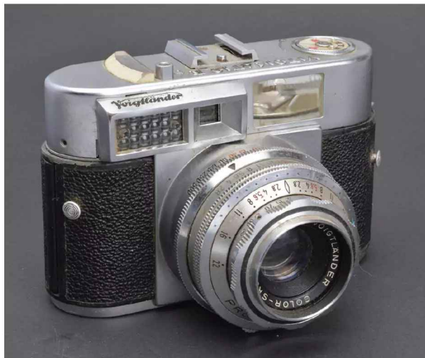
▲ Voigtlander Vitomatic IIa (1960). The Vitomatic models were compact, but very solidly-built 35mm rangefinder cameras and first introduced in 1958. The first models had a coupled selenium cell meter while later versions (from 1967) adopted a CdS meter. The IIa had a faster top shutter speed than the II (1/500 second versus 1/300 second) while there was also a run of models with a faster f/2.0 speed 50mm Ultron lens, but the camera shown here has the more common f/2.8 Skopar.
