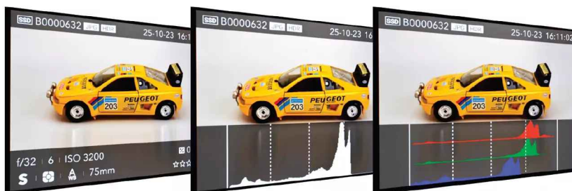
▲ Replay/review screens cycle through an info display, brightness histogram and RGB channel histograms.
