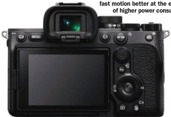
The multi-selector (better known as the joystick) is larger than previous models and plastic port covers are replaced by more durable rubber ones with seals
