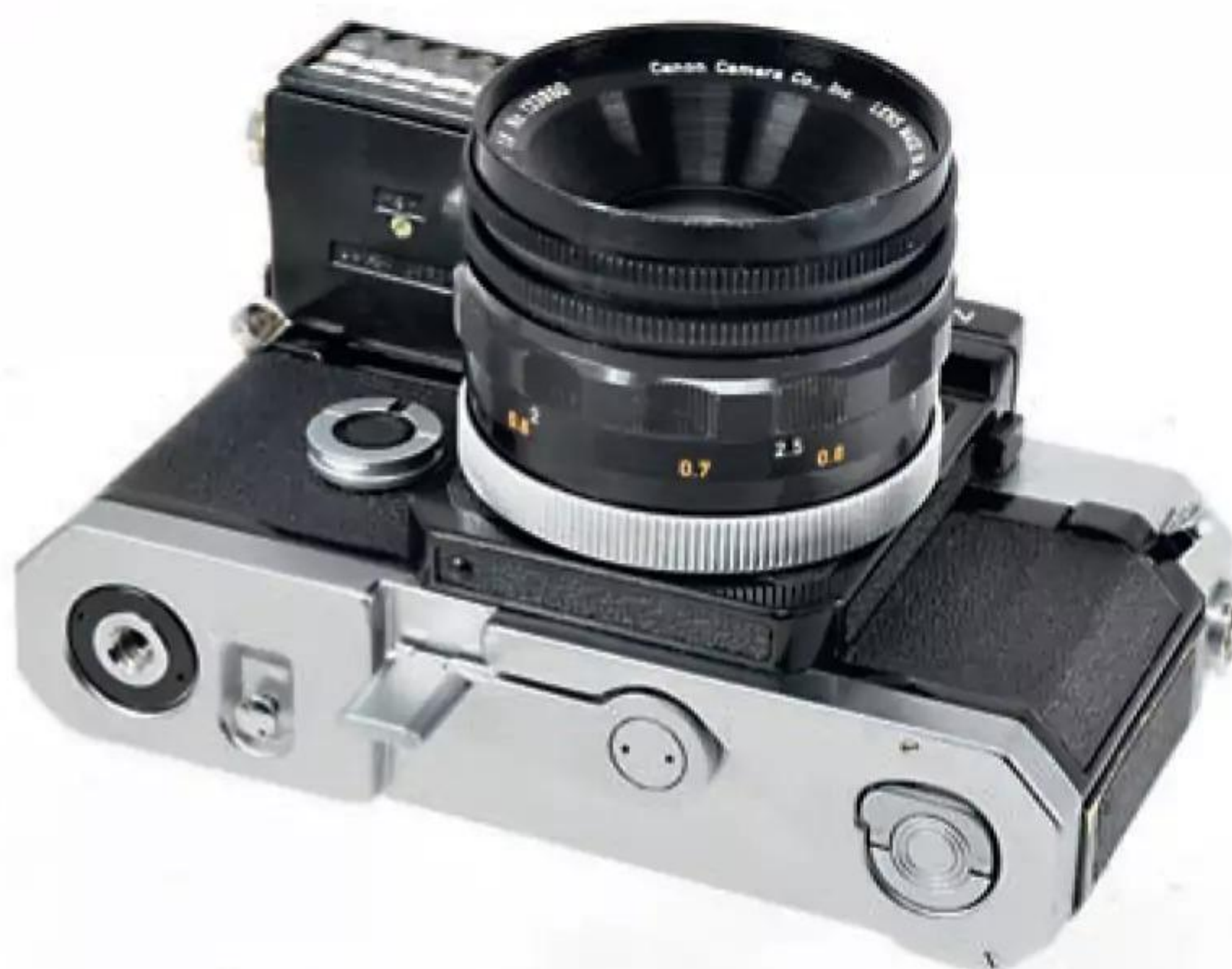
The base-mounted film wind lever on the Canonflex
