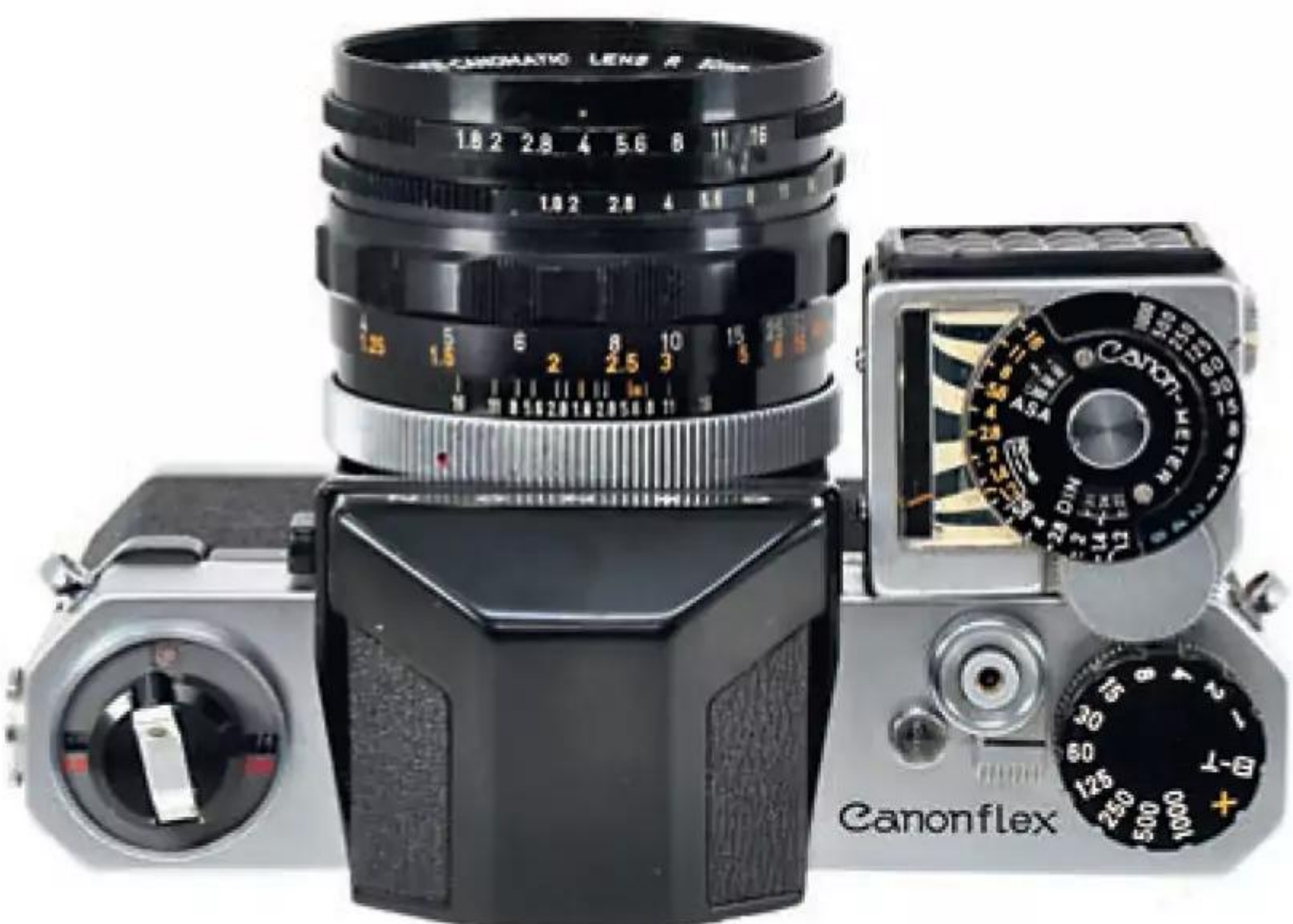
View from the top, showing how the meter connects to the shutter speed dial
