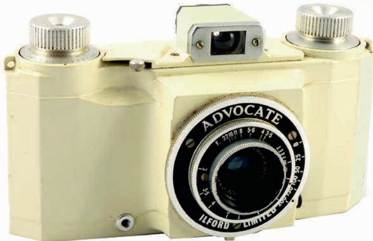
The second version of the Advocate equipped with a Wray Lustrar lens
