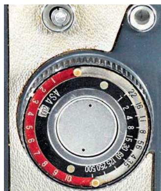
The wind knob that doubles as an exposure indicator
