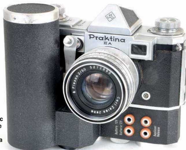
The electric motor drive fitted to a Praktina Ila
