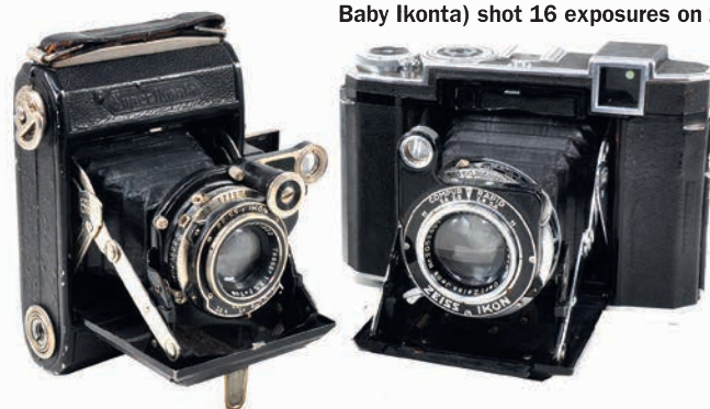
Two Super Ikontas: the Model A (left) takes 16 pictures on 120 film, the Model B shoots 11 (not 12 as might be expected) exposures on 120.
