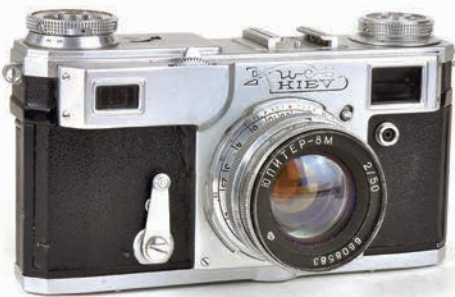
A Russian-made Kiev 4A, which was a repurposed Contax II
