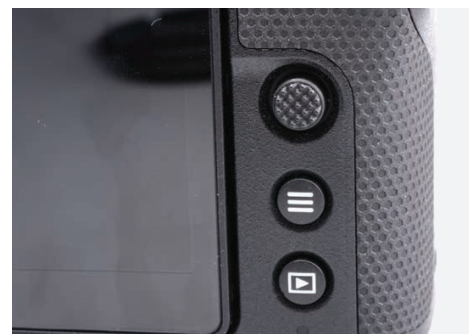
Rear control panel comprises just three buttons... the important one is the menu access button in the centre.
