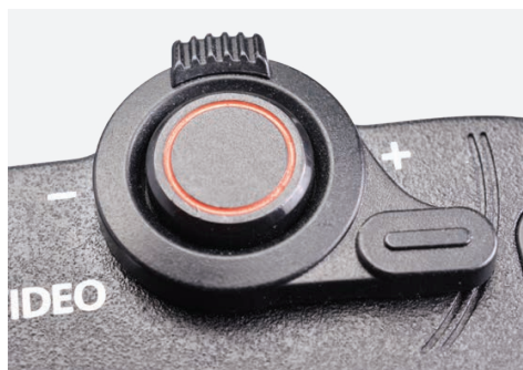
Shutter release – which is also the video/stop start button – includes a power zoom lever.
