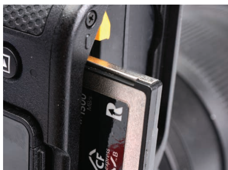
Memory card slots and battery share the same compartment in the ZR's base.
