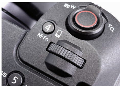
Shutter release incorporates a rocker-type power zoom control.
