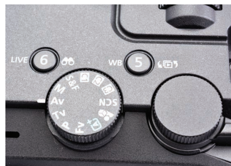
Control of the R6 V still centres around a main mode dial along with a set of three input wheels (the rear control is seen here to the right). 'S&F' position on the mode dial is for selecting slower or faster video frame rates from 1.0 to 180 fps.
