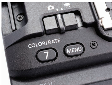
The 'Color' capture function for the 'Rate' button gives direct access to the 'Picture Style' and 'Colour Filter' menus, by-passing the main menus.
