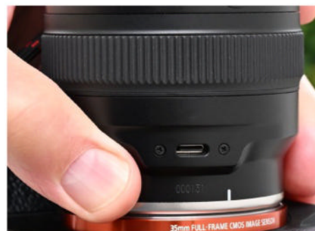
A USB-C socket allows compatibility with the Lens Utility app and Tamron-Link Bluetooth adapter.
