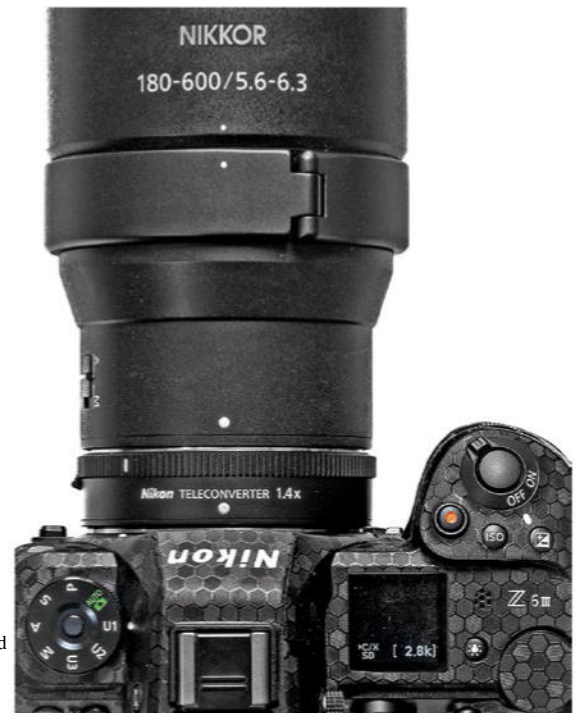
Picture 3: A TC is interposed between the lens and camera. The lens is a Nikon 180-600 mm Z Series lens.
