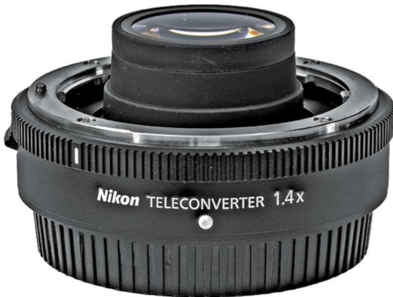
Picture 2: A sophisticated TC that supports all the functions as offered by the lens. The protruding lens elements are the reason why it cannot be used with every lens, even from the same manufacturer.
