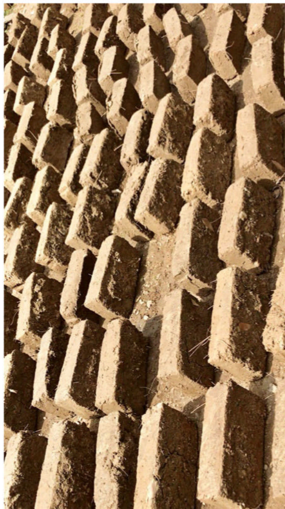
In Bir Billing, many houses are still built with bricks made with local mud and pine needles and sun dried like this
